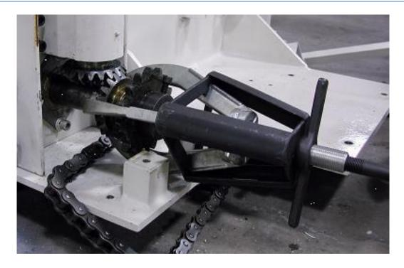
9.) Using a pulley puller, pull the gear until it is no longer meshed with the mating gear.
