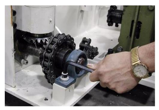
3.) Remove the 2 bolts which secure the drive shaft bearing.
