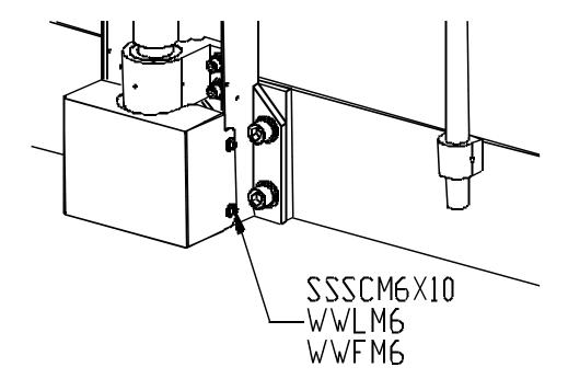
**Step 16:** Install the gear guard on the side opposite of the motor as shown above.
