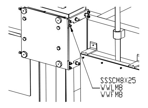
**Step 18**: Install the side guards on both sides of the machine as shown above.
