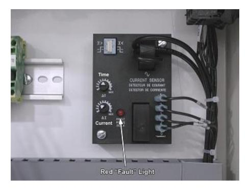
5.) Begin lowering the upper platform. If the upper platform lowers all the way until it reaches the lower limit switches without the red "Fault" light coming on there is no bind.
