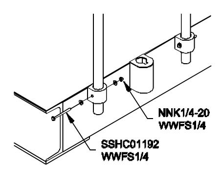
Step 14: Insert the (8) poles thru the guide rings in the top platform. Use the supplied bolts  $(1/4-20 \times 2-3/4)$  and lock nuts to secure the poles to the guide ring in the lower platform.
