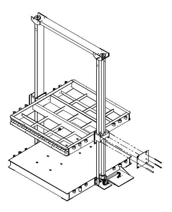
Step 8: Using the M16 X 220MM screws provided, fasten the Side Plate to the top platform. Repeat this on the other side of the machine. The screws should be torqued to  $110 \, \mathrm{lbf}$  ft.
