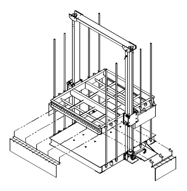
**Step 15:**Using the brackets and hardware provided, install the vinyl guards as shown above.
