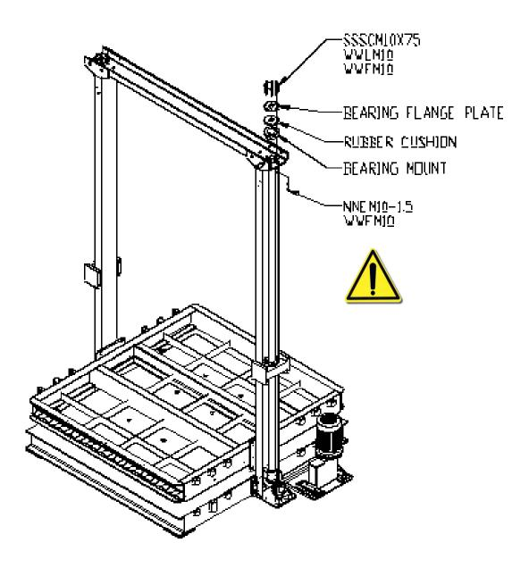
**Step 6:**Install the bearing mounts, rubber cushions and the bearing flange plates on both sides.
