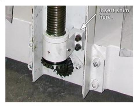
6.) After the shims have been inserted, reconnect the power source. Repeat steps 3 thru 6. Thicker shims may be required if binding still occurs.
