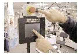
2. When the screen turns light, remove your finger and the screen will display two lines, one vertical and one horizontal, intersecting at the top left corner. The text "Touch at the crossed lines to calibrate display." should appear in various languages. In older machines, there will be no text.
