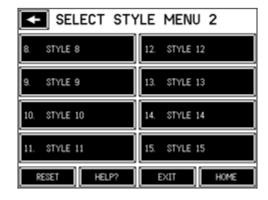
Pressing a specific style button will bring you to the style recall/edit screen. If the current security is lower than mechanic, you will only be able to recall settings. Pressing the Advanced button will allow the user to access the Advanced styles edit screen. This screen allows the user to save settings to style buttons and edit style names in addition to recalling style settings.
