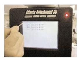
4. When the screen is touched, the display will change to two lines intersecting at the lower right of the screen.
