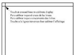
3. Using a small pointing device that will not puncture or damage the screen (such as a pencil eraser), touch the screen where the two lines intersect. Do this with as much accuracy as possible.
