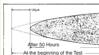
Test of Wear with a PD
